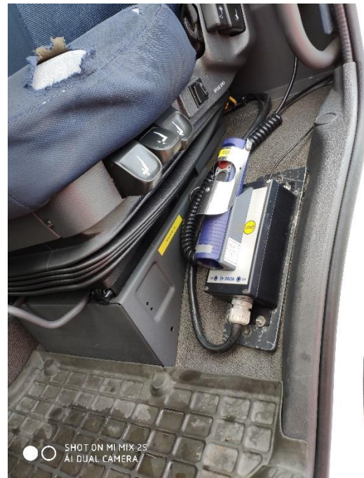
Figure 2.2 shows the position of the receiver in a tank truck for easy access. Receiver installed in this position requires normally external antenna. See section 2.5
