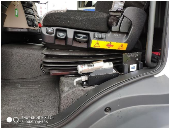
Figure 2.2 shows the position of the receiver in a tank truck for easy access. Receiver installed in this position requires normally external antenna. See section 2.5
